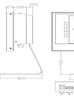
Line Drawing for: Model No. L70H All sizes are in mm Drawing not to scale.
