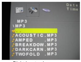
6:Press"Up/Down" Key to select the play file and press Right key to play. And press "Menu" to stop play. Then press" Catalog" return the menu. And press "Menu" into the USB Main menu.
